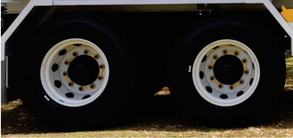
Figure 31. Wheel nut indicators must face each other
