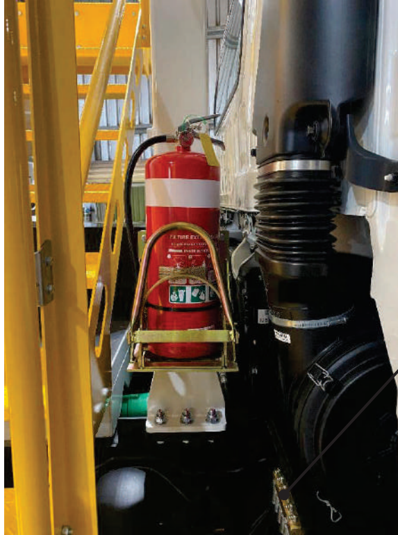
Figure 6. 9kg Fire extinguisher and grease line point behind cab on driver side.
