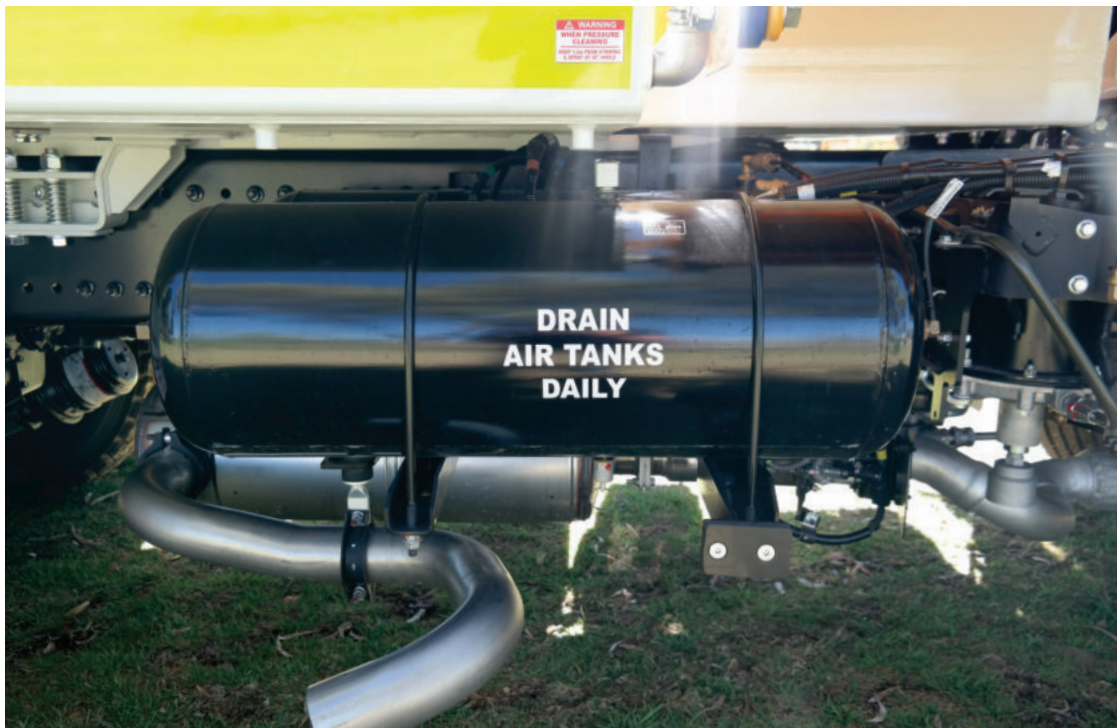
Figure 19. Air tank on the passenger side
