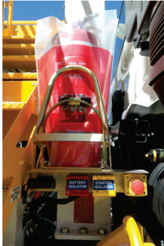
Figure 6. 9kg Fire extinguisher behind cab on driver side.
