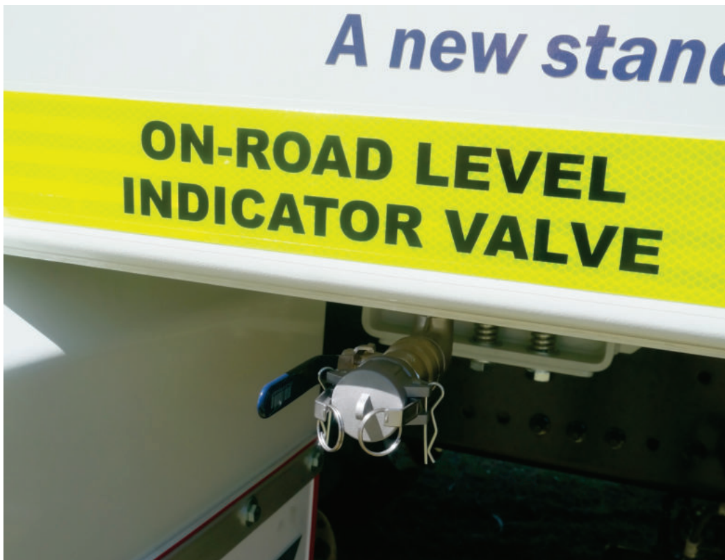
Figure 15. On-road Level Indicator Valve
