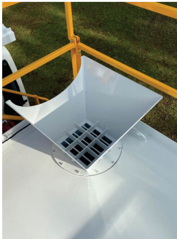
Figure 27. Funnel, relocatable to three different positions. On the driver's side by default to aid with standpipe filling.
